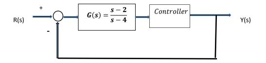
a) Determine (without computation) which of the following controller transfer functions lead to an instable feedback loop
